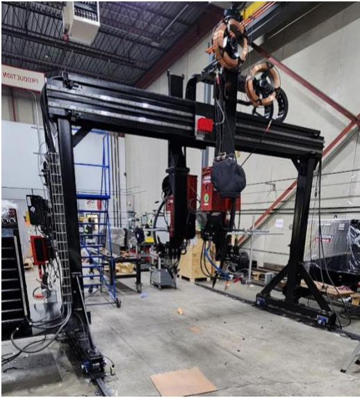
Automated SAW Gantry
